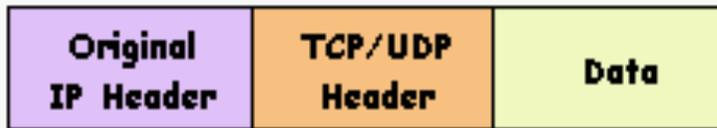
After applying ESP/UDP encapsulation
